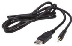
S.P.E. chargers allow to download charging cycles. In order to read these data, connect the data cable to a free USB port on the PC, switch on the charger, plug the JACK connector to the charger. At the first connection it may be required to install the software driver. For this operation, it is necessary to have a working internet connection.
